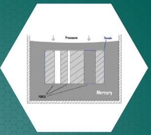
the volume of intruded nonwetting liquid are accurately measured. Combining these data with the surface tension and the contact angle of the liquid, pore diameter, pore volume, pore volume distribution and pore surface area are computed.
